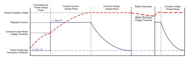
Figure 1: Current vs. Voltage Profile During Charging Phases.
