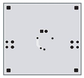
Figure 6: AAT3681 Evaluation Board Bottom Layer.
