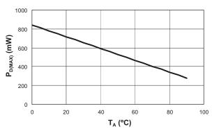
Figure 3: Maximum Power Dissipation.
