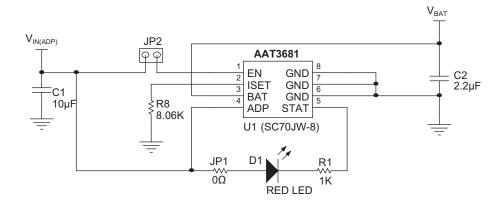
Figure 7: AAT3681 Evaluation Board Schematic Diagram.
